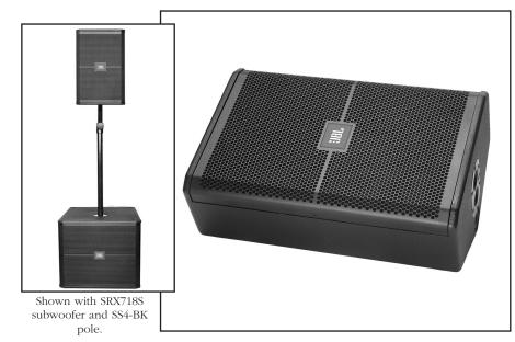
The enclosure is constructed of top quality birch plywood and coated in JBL's rugged DuraFlex<sup>™</sup> finish. The attractive CNC-machined, 16-gauge steel grille wraps around the sides of the enclosure so there are no protruding lips on the front of the box to create acoustical interference. The grilles are internally lined with acoustically transparent foam to provide additional driver protection and give a very professional appearance.
